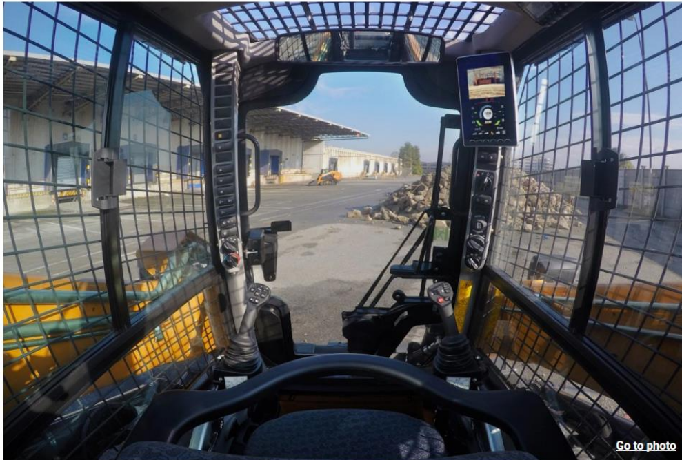
Black Hawk display by MTA mounted in CASE new B Series of loaders
