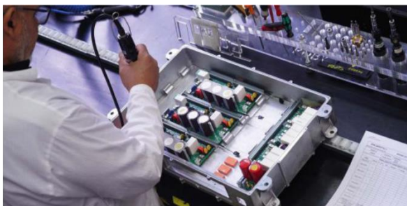
The OBC's modular design is easy to assemble to save on time and cost
