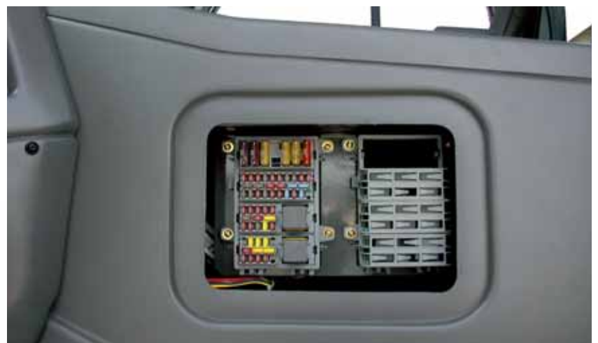
Moduli Componibili e Frame Multivie MTA Portafusibili e Portarelé MTA Multiway Frame and Modules for Fuses and Relays
