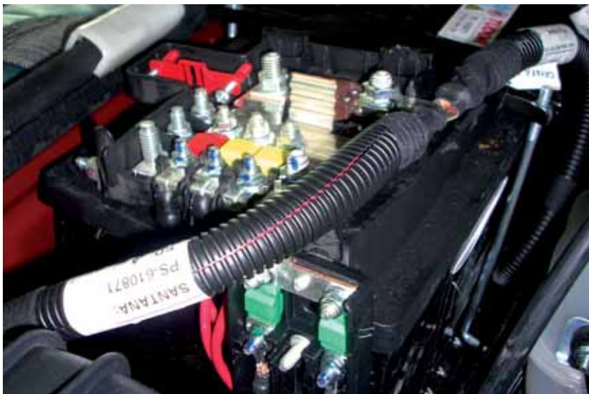
Central porta-fusíveis CBA Power e CFO Caja portafusibles CBA Power e CFO
