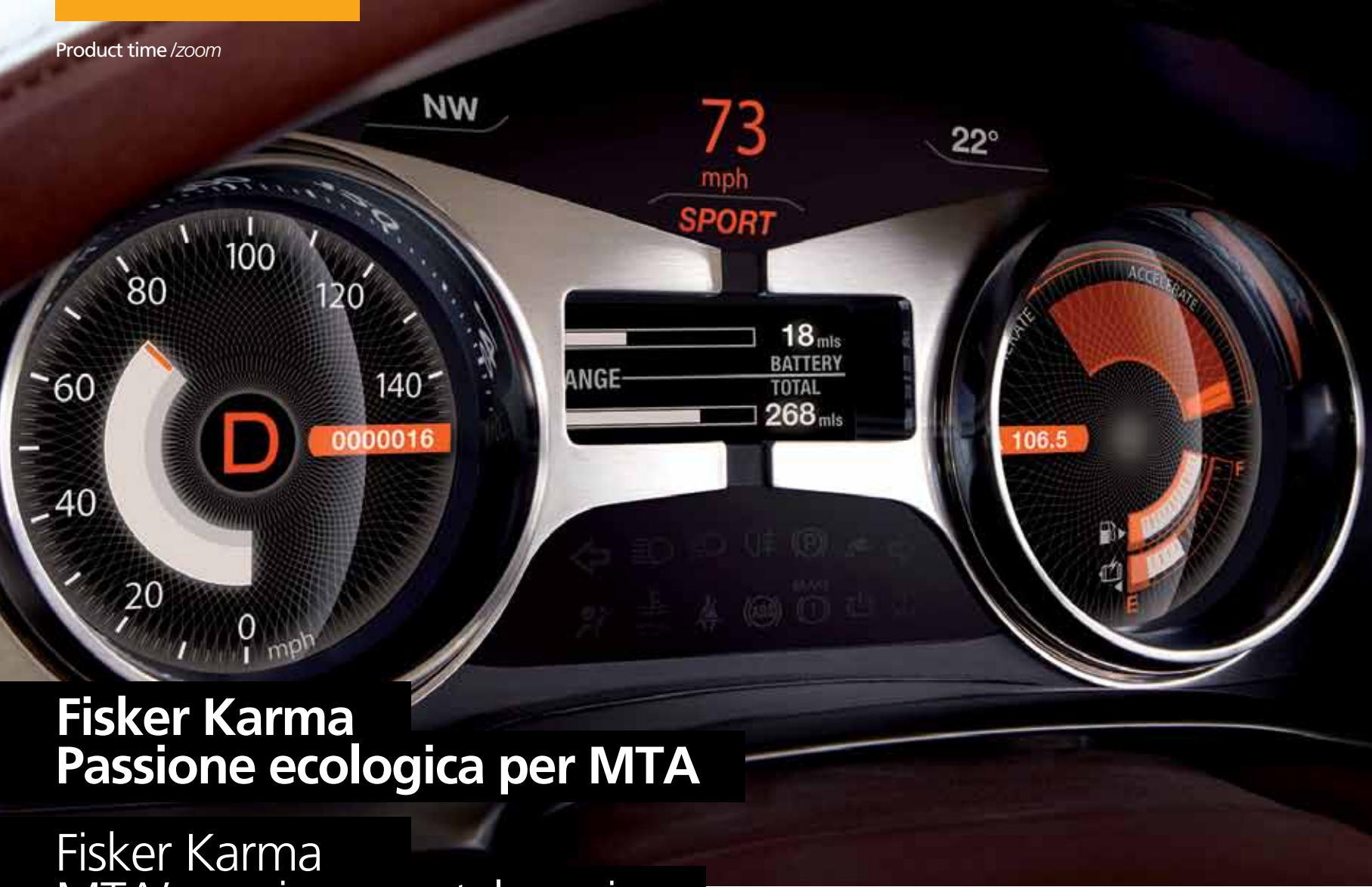
Cluster with three 5,7" TFT displays
