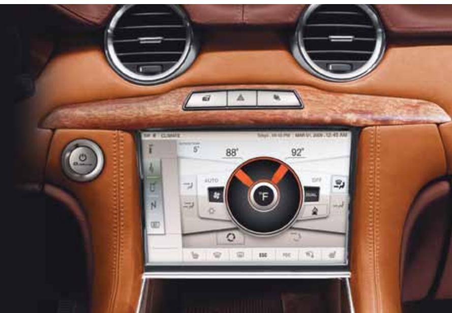
10,2" TFT Touch Panel with tactile feedback
